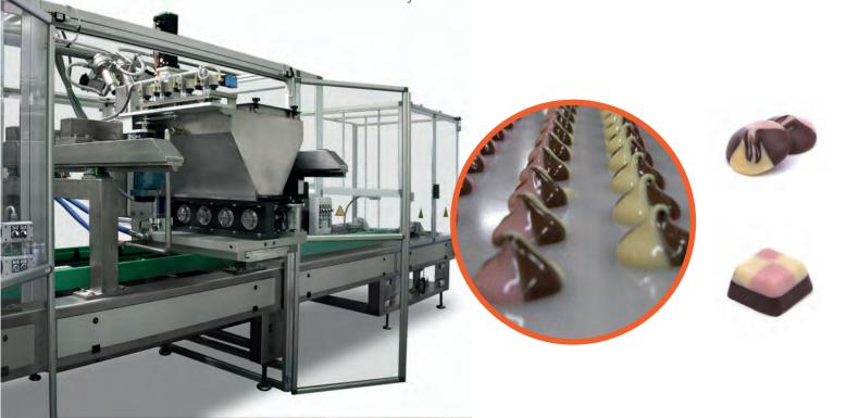
Servo-controlled piston depositors designed to guarantee maximum precision when depositing any fat, sugar-based or liquid mass, low to high viscosity, also using the one-shot system.
