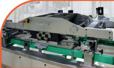
One-shot piston depositors designed to reproduce the characteristics of precision and reliability of the large Delver industrial lines on a small scale.
