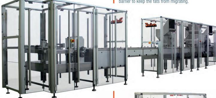
After filling and cooling, the individual products are portioned by cutting or punching the wafer sheets and separating the wafer reworks in completely automatic stations, from which the articles are directed to the enrobing or decoration lines.
